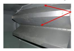
Remove the retaining bolts from around the bin divider/s to be removed and remove the divider/s.
