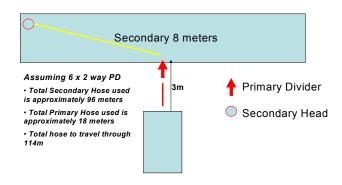
The diagram on the left shows a primary divider fitted at the centre rear of the cultivator. In this example, with a wide implement, the secondary hoses will be far in excess of the recommended five metres. In this case the primary dividers should be moved out further onto the implement, positioned as not to clash with folding, and as shown in the example below.
