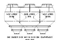
TOTAL USABLE VOLUME GIVEN A REPOSE ANGLE OF 25' IS 4692 LITRES
