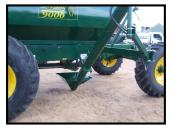
Place the auger hopper under the bin to be emptied
