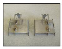
Canola covers are used to restrict spools being used to meter small seed, such as canola.
