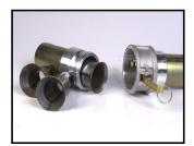
In this case air restrictors should be fitted in the line of the lighter material being sown at the lower rate. The restrictors, fitted in the male side of the camlock breakaways as shown, simply restrict the air flow, stopping the escape of air and keep the system in proper balance.
