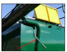
**Step 3**Place auger on the front mount and secure by returning the latch
