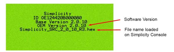
The above screen is displayed for 60 seconds each time the Seeder Console is switched on using the 'power' switch. It is not necessary to have this information displayed for the full 60 seconds if not required. When the screen is displayed simply push the 'enter' button to move into the working screen.
