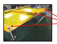
Further adjustment is available by tightening the lock nuts on the hinges.
