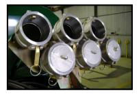
Disconnect primary lines not in use at the breakaway connections on the air seeder. Fit camlock blanking plugs to the lines not being used so that air cannot escape.
