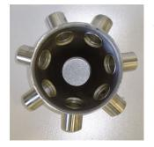
The Secondary Head is manufactured from stainless steel and has either a 44.5mm, 50mm or 63mm internal diameter inlet depending on the uptube and can have 4 to 10 outlets per head. The outlets are 32.5 mm outside diameter to accommodate the terminal lines. The Secondary Head is sealed at the top by a durable rubber cap to avoid seed damage.
