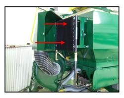
The hydraulic oil cooler fitted to all Simplicity Airseeders should be periodically checked and cleared of trash build up.
