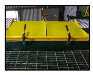
When closing the lids check that the latches close with 'over centre' force. This will ensure that the lids are tight and pressure is applied to the seal.
